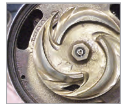
Competitor Impeller is effectively worn out.
